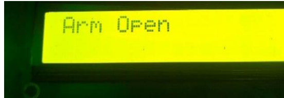
Fig. 10. LCD display showing robotic arm opening operation
