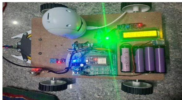
Fig. 8. Experimental prototype of the proposed bomb sensing robotic platform
