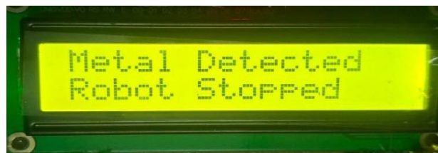
Fig. 9. LCD display showing metal detection alert message
